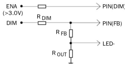
ENA voltage > 3.0V; output current increases as DIM voltage decreases
